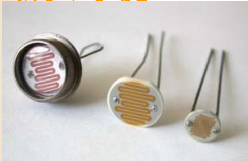
Photocell (light sensor)
